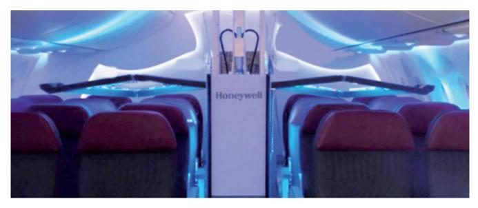
UVC disinfection works by exposing material surfaces to Ultra Violet light that falls in the region between visibile light & X-rays:
