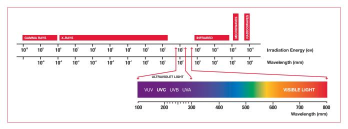
The short wavelengths of ultraviolet light inactivate microorganisms by destroying nucleic acids and disrupting their DNA, leaving them unable to perform vital celluar functions. Wavelengths between 200 and 300 nm when exposed to microorganisms cause defects which prevent cell replication and can lead to inactivation of the organism.
